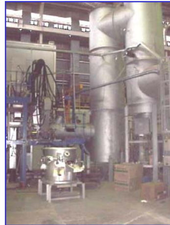
Plasma inertization reactor (left) e post-combustion camera (right) of the CSM 500 kW Plasma Torch Pilot Plant
