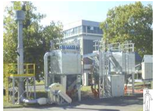
■ Process Module 1 – ACW feeding system, torch reactor, post-combustor and quencher
