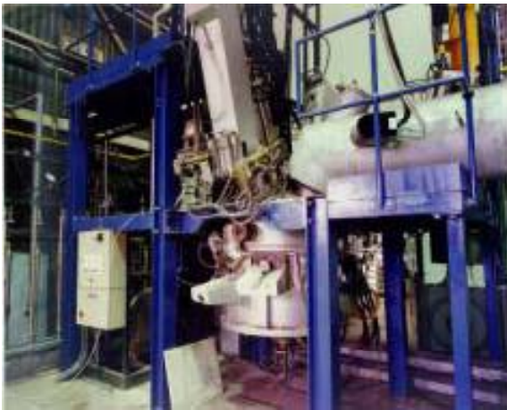
Plasma inertization reactor (left) e post-combustion camera (right) of the CSM 500 kW Plasma Torch Pilot Plant
