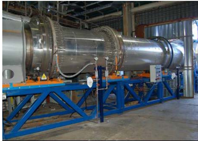
Feeding system (left) and process reactor (right) of the CSM rotary kiln gasifier pilot plant
