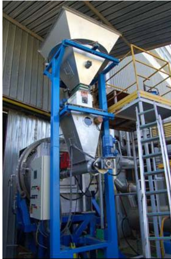
Feeding system (left) and process reactor (right) of the CSM rotary kiln gasifier pilot plant
