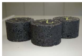
Samples of bituminous conglomerate produced using GRANIMIX® and used in environmental and technological tests.
