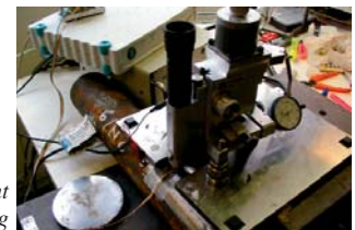
Residual stress measurement device by Hole Drilling
