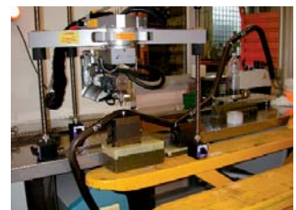
Sachs method - Steel pipe internal diameter boring out.
