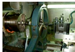
Residual stress measurement device by Hole Drilling
