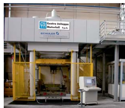
CSM's Semi-Industrial Hydroforming Press for Sheet and Pipes (3000 tons, 4000 bars)
