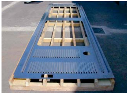
Component of side panel laser welded
